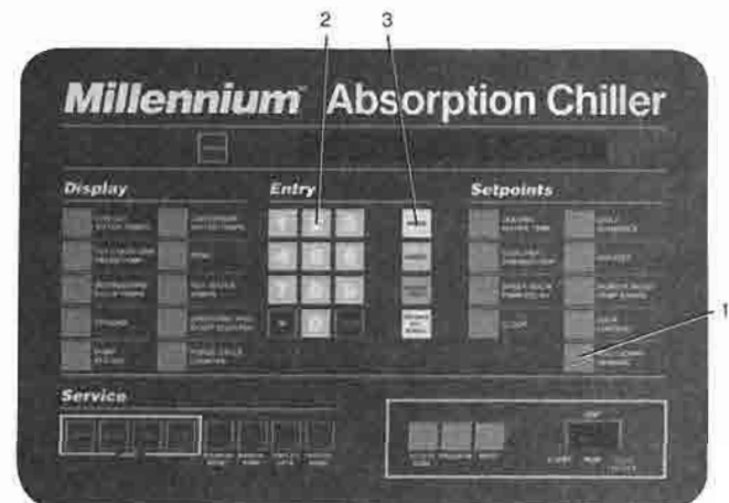
FIG. 11 - KEYPAD - PROGRAMMING "PULL DOWN DEMAND" SETPOINT
